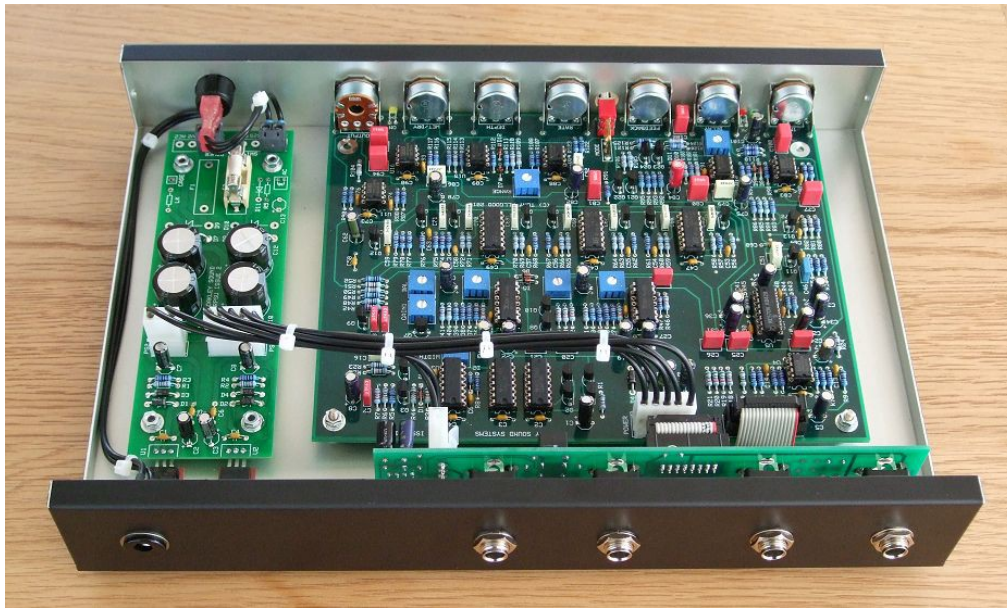
The prototype ADR30 built into a low cost Takachi YM-300 project case. The unit is powered from an external 500mA 15V AC wallwart keeping all high voltages out of the case.
