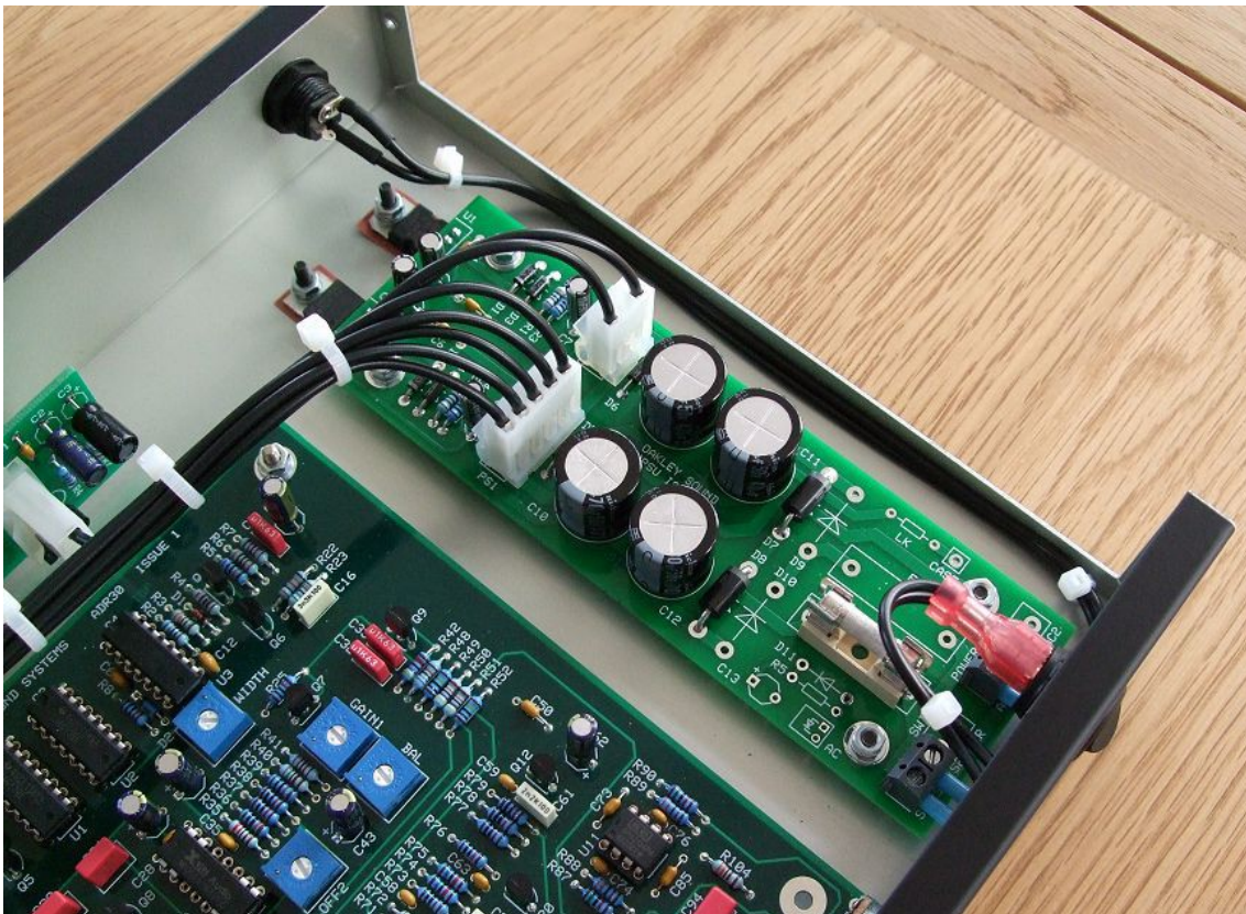
The issue 2 RPSU board fitted to a Takachi YM-300 case. The RPSU has been built in the recommended half-wave option suitable for powering a single ADR30 main board.
