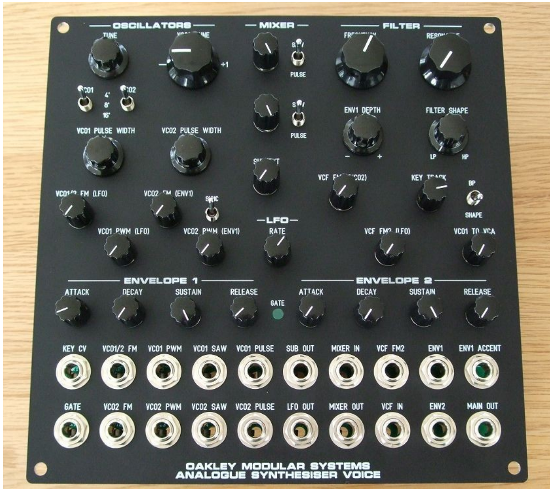
The first prototype unit using a printed Schaeffer panel. The nuts for the switches have not yet been fitted.
