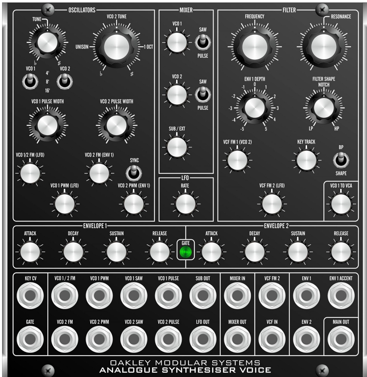
The suggested panel design for the 4MU wide MU format module.
