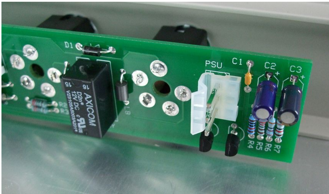
The relay and power muting circuitry on the SREIO board.
