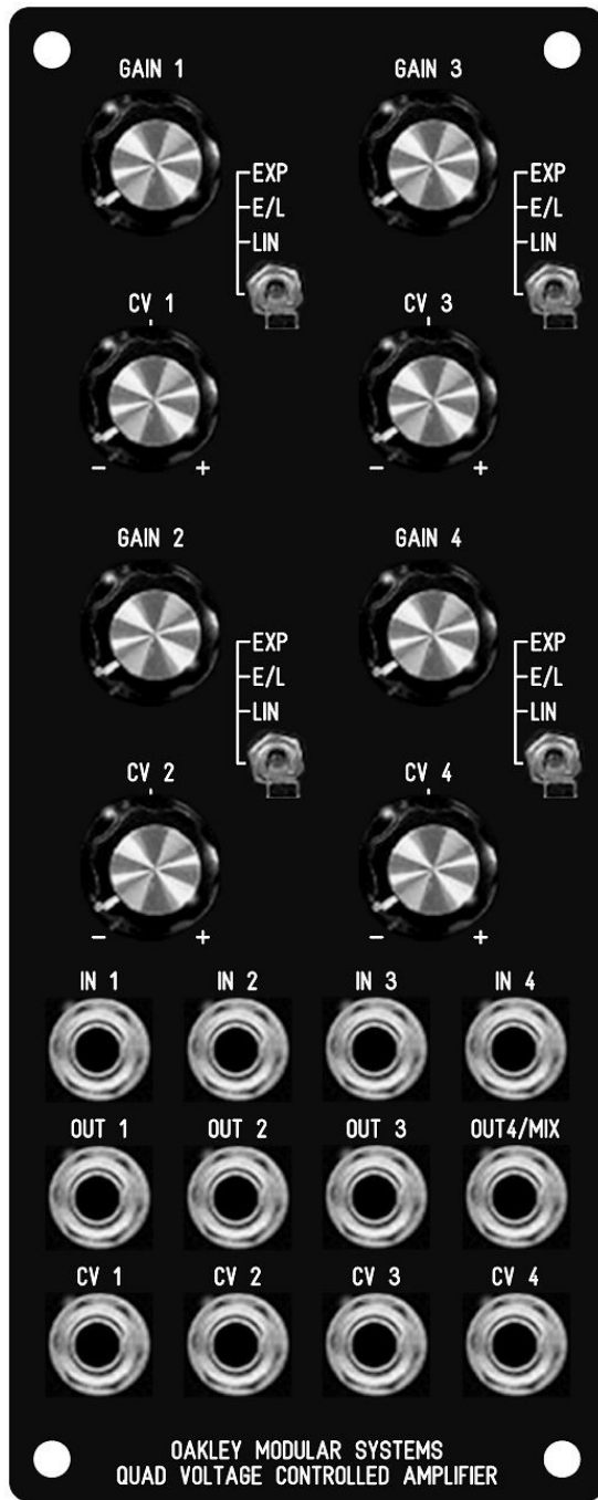
The suggested panel layout for the dual width MOTM format module.
