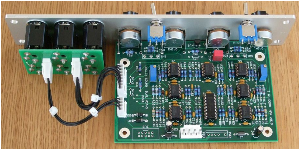
This is the Oakley Dual VCA module built with the issue 1 Dual VCA-X PCB behind a natural finish 1U wide Schaeffer panel.
