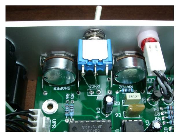
*This is an Apem SPDT (on-on) toggle switch. Note that for both switches it is the lower two tangs of the switch that connect to the PCB.*
