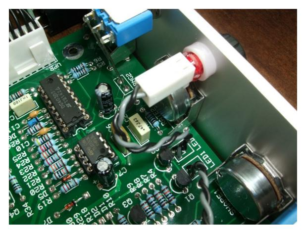
Here I have used a Molex 0.1" KK header and crimps to attach the LED to the PCB. The LED is thus not soldered to the wiring allowing the board to be easily removed from the front panel.
