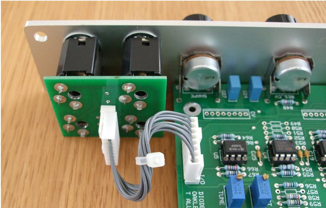
*The prototype Diode Superladder filter core module showing the detail of the board to board interconnect. Here I have used the Molex KK 0.1" system to connect the Sock4 to the main PCB.*
