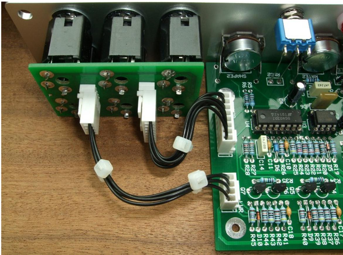
*The Sock6 board makes it much easier to build the module. Here I have used Molex 0.1" KK headers and housings. This is a 'strip and crimp' system that is cheap but very reliable.*
