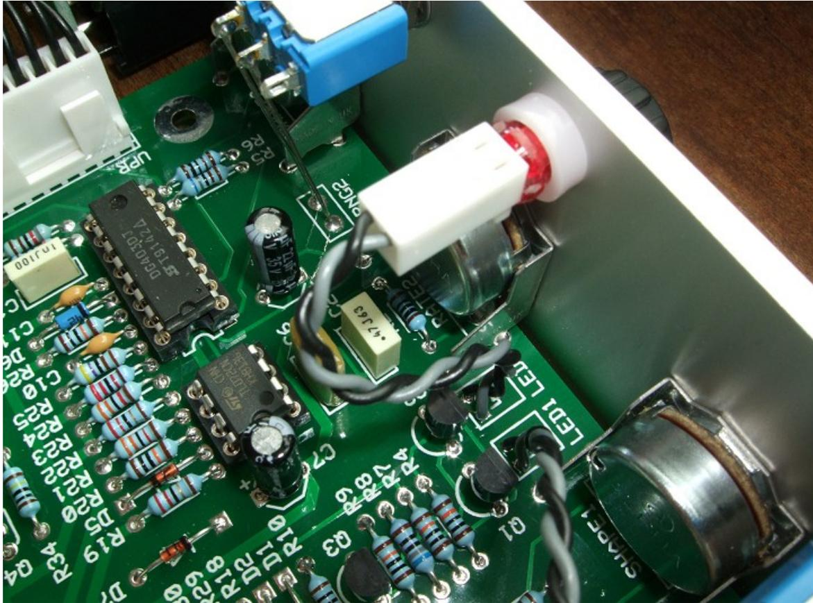
*Here I have used a Molex 0.1" KK header and crimps to attach the LED to the PCB. The LED is thus not soldered to the wiring allowing the board to be easily removed from the front panel.*
