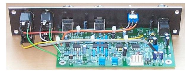
There are four sockets, one switch and three LEDs in the new suggested EFG layout. The later versions of the suggested layout now makes the preamplifier output available, but looses the simultaneous slow/fast outputs in favour of a switch. The preamplifier still drives the envelope follower directly.
