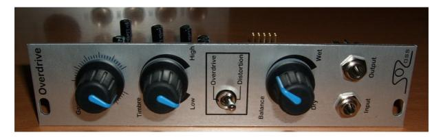
The Oakley Overdrive module for the Eurorack format. This module has been built by Krisp1.
