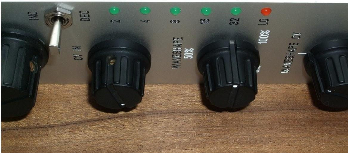
*Using a 3mm thick panel the domed top of the LEDs just sit proud of the panel surface giving a neat appearance.*
